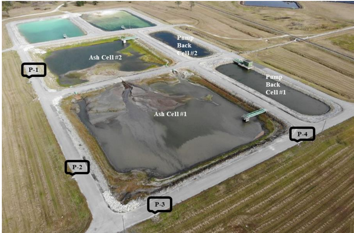
Figure 1. Layout of the CCR Surface Impoundment System and Adjacent Pump Back Ponds (Picture was taken by ITS on 20 December 2019)
